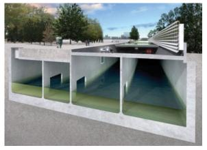
One strategy cited for on-site storage is the use of underground parking garages. Please note that when this strategy is used, the water storage area is typically separate from the parking area, as shown in the depiction of a stormwater storage tank built under a parking garage in downtown Rotterdam (see left).
