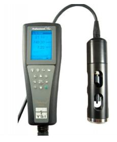
conductivity reading (the  $\mu$ s/cm screen with °C symbol flashing). The reading should be within  $\pm$  10% of the standard or 20 uS/cm (whichever is greater). If it is not, the meter will need to be calibrated with the standard, according to (Pgs. 12-13 of) the manufacturer's instructions. Rinse the probe well with de-ionized water or tap water before reinserting it into the chamber.
